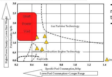
Future MALE design space powerplant not typically addressed by either gas turbine or piston engine systems.
