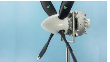
•Siemens new prototype electric motor specifically designed for aircraft that weighs in at just 50 kg (110 lb) and is claimed to produce about 260 kW
